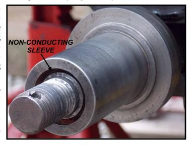
Now that the wheels are off, start cleaning everything really well. Blow out bearings and rewash as needed until they are nice and clean and turn freely. Clean the bores of the hubs out and inspect bearing for pits, flaking, scoring and any other surface defect, you know what a good race looks like. Be very careful because the machined-in-hub labyrinth seal grooves are sharp and will cut fingers!
