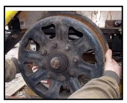
Remove cotter pin and castle nuts from axle. Remember these are right hand threads so righty-is-tighty and lefty-is-loosy. The wheel bearing hub assembly should slide off but if it won't, a few solid blows to the back of the wheel with a soft face, dead-blow hammer will get it moving. If not, a 3 jaw puller may be used.
